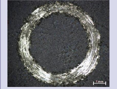
The wear pattern of the coating t ano 10 500 clearly shows that the coating is completely detached during abrasion, and that a distinctive form of abrasive wear, the so-called abrasive wear, is applied to the soft, metallic substrate. traces of microfabrication wear [2] are visible
